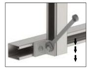
5. Using a wrench to tighten the bolt will lock the serrated teeth of the channel nut onto the inturned edges of the channel.
