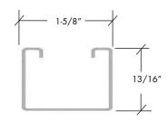
Channels are accurately and carefully cold rolled formed to size from low-carbon strip steel. Cold rolled and stainless steel are offered only 16 gauge.
