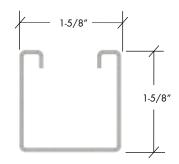
Channels are accurately and carefully cold rolled formed to size from low-carbon strip steel. Cold rolled and stainless steel are offered in 12 gauge.
