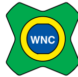
Non-Potable Water, Cold
