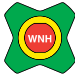
Non-Potable Water, Hot
