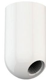
BI148-2S-VR Extended overhead mounted wye fitting. 3/8" NPT female inlet, (2) 3/8" NPT outlets at 90 degrees.
