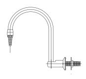
**Application:** Panel mounted gooseneck for use with foot-operated valve.
