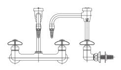
**Application:** Panel mounted faucet for hot and cold water with horizontal inlets on 8" centers.
