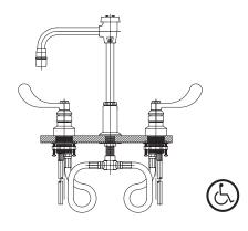
**Application:** Deck mounted faucet with vacuum breaker on 8" centers for hot and cold water.
