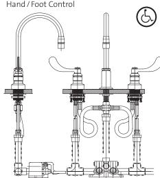
**Application:** Deck mounted mixing faucet with floor mounted pedal valve. Faucet may be actuated by either faucet handles or foot pedals.
