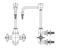
**Application:** Panel mounted faucet for hot and cold water with vertical inlets. Inlets are on 3" centers, cold water on bottom.
