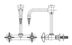
**Application:** Panel mounted faucet for hot and cold water with horizontal inlets on 6" centers.
