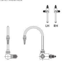
**Application:** Panel mounted faucet for distilled, deionized or reverse osmosis water. Faucet has exterior brass casing and interior lining of inert polypropylene. Pure water comes in contact only with inert plastic.
