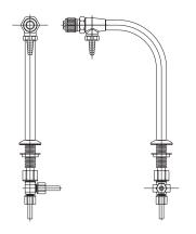
**Application:** Deck mounted faucet for distilled, deionized or reverse osmosis water. Faucet is fully recirculating to eliminate all "dead legs" in pure water system.
