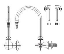
**Application:** Panel mounted faucet for distilled, deionized or reverse osmosis water. All components in contact with water have interior lining of pure tin.
