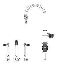
**Application:** Deck mounted faucet for distilled, deionized or reverse osmosis water. Faucet has exterior brass casing and interior lining of inert polypropylene. Pure water comes in contact only with inert plastic.
