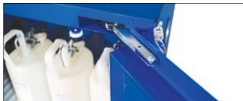
Encased self-closing mechanism provides obstruction-free access to top shelf space. Fusible link melts at 165°F (74°C) to automatically close door(s) under fire conditions.
