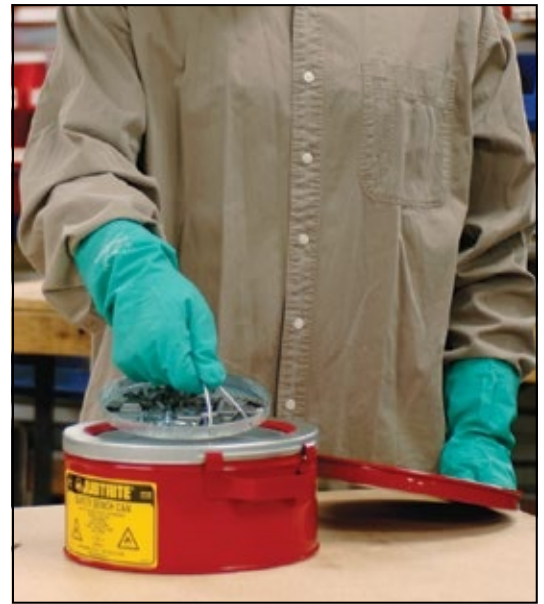
Clean small parts by pushing down dasher plate and agitate in cleaning solvent.
