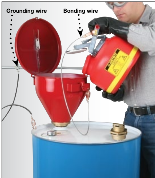
Proper bonding and grounding techniques prevent static discharge and the potential for fire.
