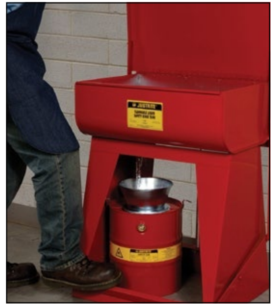
Position drain cans under rinse tanks to safely collect used solvents.
