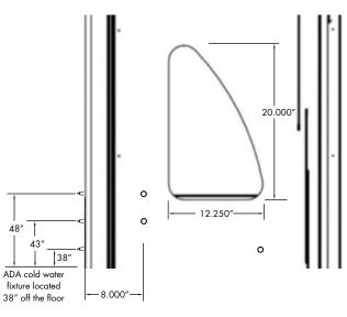
NOTE: Standard fixture location (not ADA) is 39-3/4" off the floor and are spaced 5" apart for standard applications.
