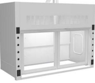
**Counterbalance Systems** - Chain and sprocket system delivers the easiest and most reliable sash operation available with an exceptionally long life span. High quality stainless steel cable system provides economical and reliable operation; tested to 100,000 cycles with no failure.
