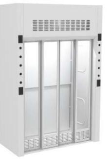
**Sash Design** - 6mm laminated safety glass is provided with a stainless steel handle and side runners, optional tempered glass or polycarbonate available for special applications. Hoods are supplied with horizontal sliding sashes. Floor mounted fume hoods are designed to operate with only one sash open.
