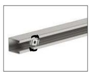
2. Turn clockwise 90° to line up the grooves in the nut with the inturned edges of the channel.
