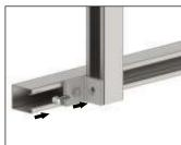
4. Added channels are able to be bolted to the existing fitting by following procedure described in steps 1-3.
