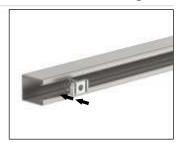
1. Place the spring nut anywhere along the continuous slotted channel.
