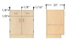
☐ Full Flush Overlay (Standard) Feature square-edged door and drawer fronts with tight reveals by notching around the hinge
