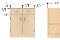
☐ Reveal Overlay Feature square-edged door and drawer fronts with no hinge notching on the doors providing balanced reveals
