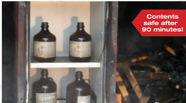
Contents remain intact after a 90-minute burn test.
