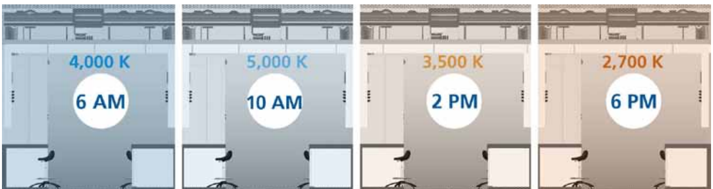
Figure 1 – This generic example shows how the lighting temperature and intensity could be programmed throughout the day to match the rhythm of the sun. This indoor 'Biodynamic Light' is an available option that is said to set the body's circadian rhythm, which brings health and comfort to the workforce.
