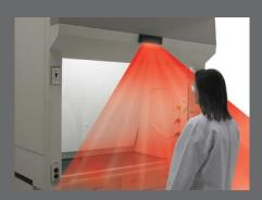
Overhead Presence Sensor - Monitors the work area in front of the fume hood to detect the presence of the user. When the user stands in front of the fume hood the sensor will automatically open. Sash closes when the fume hood is left unattended after a set time delay. The closing time delay is adjustable on site.
