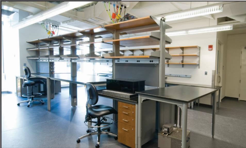
**2500 Series** - Sturdy 6" wide obround frames with tubular legs and leveling feet are 84" high. Modular design allows for several systems to be connected together to create custom assemblies with services being fed throughout each unit. Services are easily accessible by removable panels on the leg posts. Bench units are available in 48", 60", 72" and 96" widths.
