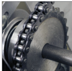
Chain and sprocket sash
