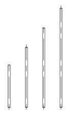
3/4" diameter vertical rods are machined with the top end rounded and the bottom end tapered to fit into a rod socket. 1/2" diameter vertical rods are machined with the top end rounded and the bottom end threaded. 1/2" rods may be used either with a threaded socket or with the AAP120 tapered adaptor and a tapered socket.
