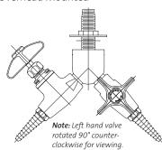
**Mounting:** For installation on vertical or horizontal surfaces (such as pipe chases and service carriers) where there is access behind surface during installation.
