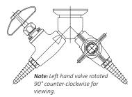
**Mounting:** For installation on vertical surfaces (such as drywall) where there is no access behind wall during installation.
