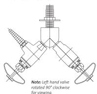
**Mounting:** For installation on vertical or horizontal surfaces (such as pipe chases and service carriers) where there is access behind surface during installation.
