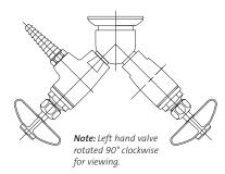
Mounting: For installation on vertical surfaces (such as drywall) where there is no access behind wall during installation. Wye fitting is threaded onto nipple stubbed out of wall. Threaded escutcheon is then backed up to wall to secure fixture and conceal pipe.
