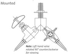
**Mounting:** For installation on vertical or horizontal surfaces (such as pipe chases and service carriers) where there is access behind surface during installation.
