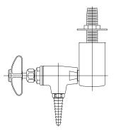
**Mounting:** Turret base with single outlet for mounting underneath reagent shelf.
