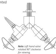
Mounting: For installation on vertical or horizontal surfaces (such as pipe chases and service carriers) where there is access behind surface during installation. Threaded mounting shank is inserted through hole in surface and secured with locknut and washer.
