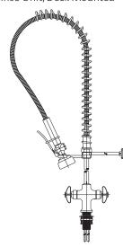
**Application:** Deck mounted pre-rinse unit for hot and cold water.
