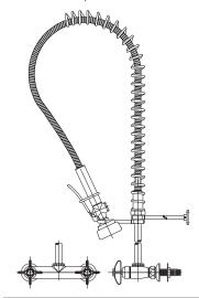
**Application:** Panel mounted pre-rinse unit for hot and cold water.
