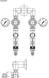
**Application:** Low pressure point-of-use regulation of carbon dioxide and high purity gases. Used for supplying CO2 to incubators, low pressure compressed air applications and low pressure inert high purity gases, including nitrogen, helium, argon and oxygen.
