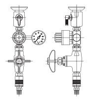
**Application:** Point-of-use regulation of high purity gases. Used for compressed air and inert high purity gases, including nitrogen, helium, argon and oxygen. Pressure regulator has elastomer diaphragm and O-ring seals.
