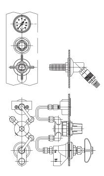
**Application:** Point-of-use regulation of high purity gases for installation on fume hoods. Used for compressed air and inert high purity gases, including nitrogen, helium, argon and oxygen.
