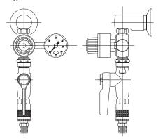
**Application:** Low pressure point-of-use regulation of carbon dioxide and high purity gases. Used for supplying CO2 to incubators, low pressure compressed air applications and low pressure inert high purity gases, including nitrogen, helium, argon and oxygen.
