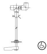
Application: Remote control ball valve for water and gases. Valve is mounted in horizontal position within side wall or underneath deck of hood. Valve provides on / off control of service, is certified for natural gas service by CSA International and is recommended for ADA-compliant applications. Furnished complete with anodized aluminum extension rod, guide plate and handle.
