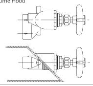
**Application:** Panel mounted valve for installation on angle face of hood. Valve is installed from behind panel and is secured with 45 degree angle escutcheon and external locking ring on front of hood. All working components of valve are accessible from front exterior face of hood.
